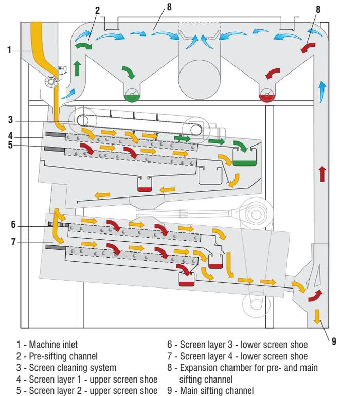
The purpose of the **PETKUS U-Cleaner** is the high-quality cleaning of grain, pulses, oilseeds and other free flowing products. The cleaner can be used for pre-, intensive and seed cleaning. The high standard of cleaning is achieved by a combination of the screening process and the air aspiration system.
