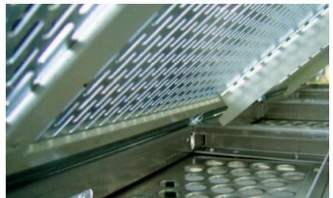
Screensegment within exchangeable screen frame
