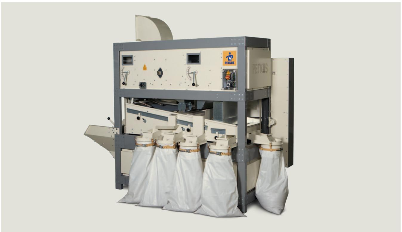
The **PETKUS Seed Cleaner K 06** is used for high-quality seed cleaning of free flowing bulky products, e.g. pulses which do not need to be processed with an indented cylinder. Furthermore, the seed cleaner can also be used for the intensive cleaning of grain and oilseeds. The high standard of cleaning is achieved by a combination of the screening system and the air aspiration.
