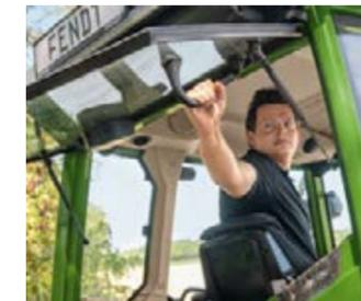
A special feature of the Fendt 200 Vario is the vertical handle on the rear window, which lets you open and close the window from the comfort of your seat.
