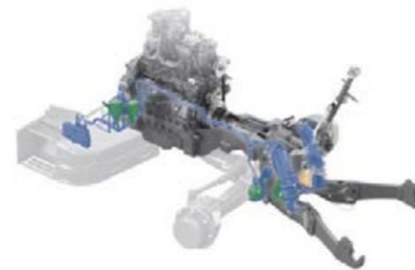
The front power lift is fully integrated and sits tight against the vehicle. This keeps the linked machines highly manoeuvrable. The lower links have a low bottom grip and can be folded for parking. Bellows protect the lifting cylinders against stone impact. The vibration damping fitted as standard prevents bounce and guarantees safe driving and comfort.
