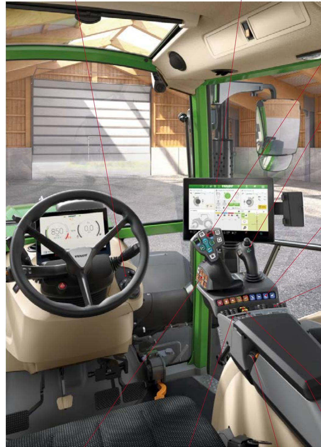
As well as the familiar clover leaf operation, the new multifunction joystick includes two controls for proportional valve control as well as four freely assignable white keypads.
