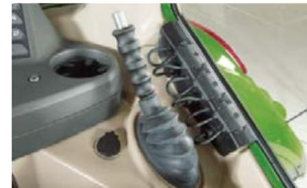
Fendt offers a clever solution for cables that run from the rear of the tractor into the cab. Cables can be guided through the lead-through, no matter what kind of cross section they have. The rear window can be closed, so dust, dirt, water and noise stay outside.
