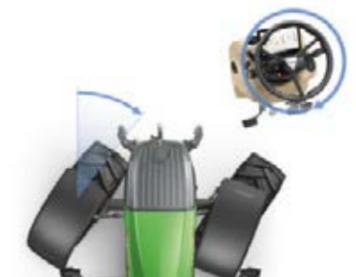
At the headland or during front loading work, you benefit from FendtActive steering\*, reaching a full wheel turn with just one steering wheel rotation. Up to 8 km/h the superimposed steering system is unrestricted, from 8 to 18 km/h the superimposition effect is linear.
